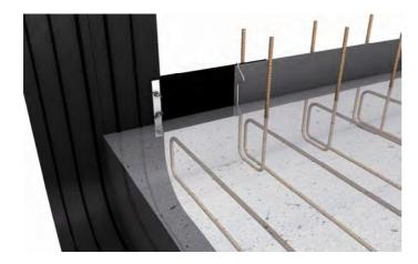
The wolfseal expansion joint connection is placed at the desired position of the expansion joint band. The holes are done from the water exposed side with a hole punch and screw together with the expansion joint band.
